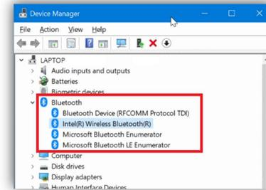
If the Bluetooth category exists in the Device Manager window similar to the above image then you likely do have an internal Bluetooth adapter present in your computer. If not then you do not have that feature and may proceed by inserting the USB Bluetooth adapter to your computer and allow time for it to be recognized by Windows and for its device drivers to be automatically installed. You may then skip to section 1.1.2 below.
