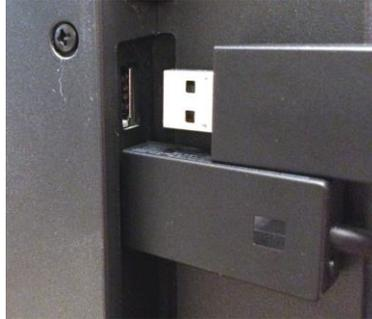
3. Otherwise, you may need to find a USB wall adapter such as what might come with a smart phone. Plug the USB end of the Wireless Display Adapter into the USB wall adapter and then plug that adapter into a wall outlet.
