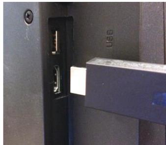
2. If you have an available USB port in the back of your TV or external display then plug the USB end of Wireless Display Adapter into this port
