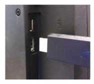
2. If you have an available USB port in the back of your TV or external display then plug the USB end of Wireless Display Adapter into this port
